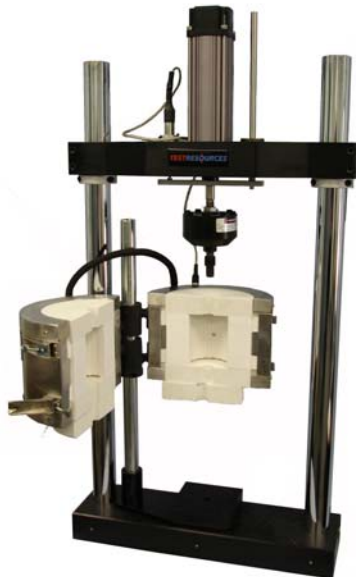
800RE3 – static and cyclic tests on ceramics within a 1000C furnace
